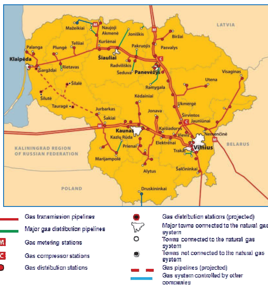
Figure 3.6.5.1-1. Gas distribution network in Lithuania
