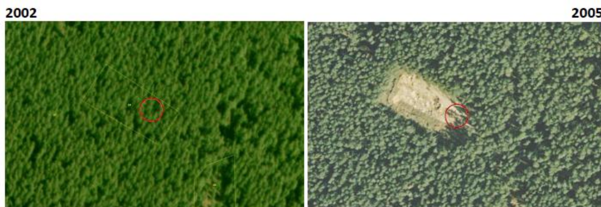
Figure 11-2. Identification of deforestation (D) case using two consecutive orthophotos
